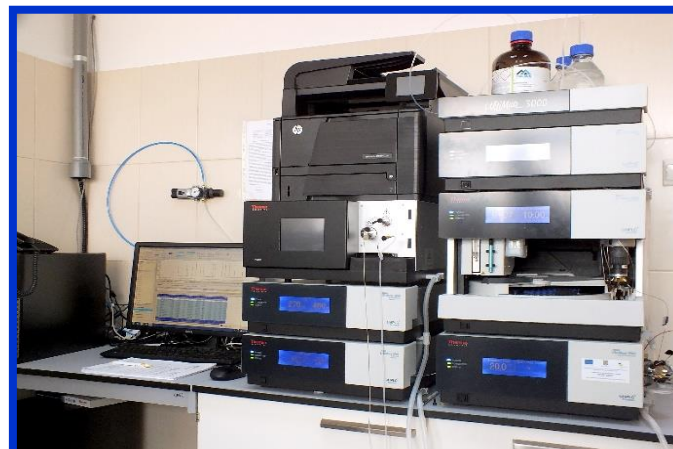
HPLC cu detector fluorescenta
